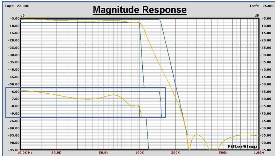
After the Max constraint is edited, and the circuit reoptimized, the results below are produced. This time the error was reduced to zero and the circuit response is contained entirely within the constraints.
