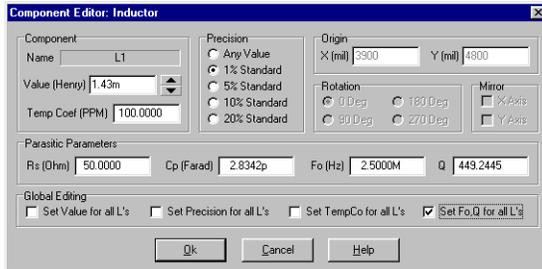
All of these parameters are considerably worse than those of the previous axial component. As before we will assume that the AC resistance at 100kHz will be slightly larger than the DC value, say 50 Ohms.
