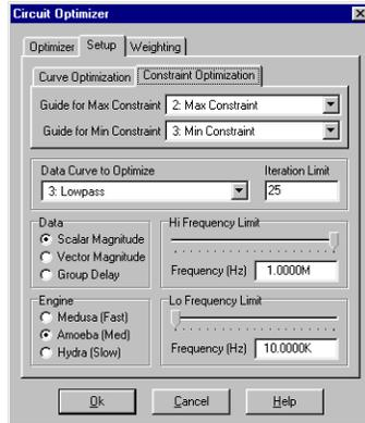
Eight components are selected for optimization including all L/C values and R1. R2 is not optimized to prevent the entire impedance of the circuit from sliding.
