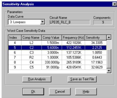
The *Sensitivity Analysis* now shows some very large values for a few of the components. Noting the frequencies, we can see that these values occur at the location of the zeros. The zeros of an Elliptic type response cause difficulty for evaluating sensitivity.
