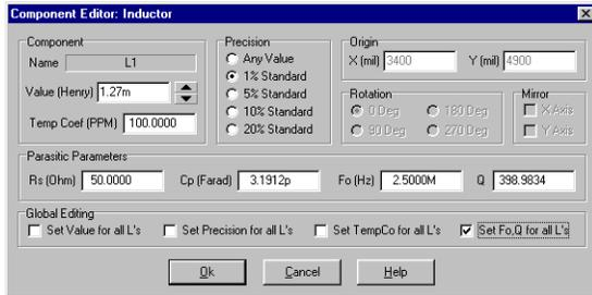
After the inductors are edited with the values  $F_o=2.5\text{MHz}$  and  $R_s=50\text{ Ohms}$ , and the circuit recalculated, the response shown below is produced in Yellow and the target in Black.
