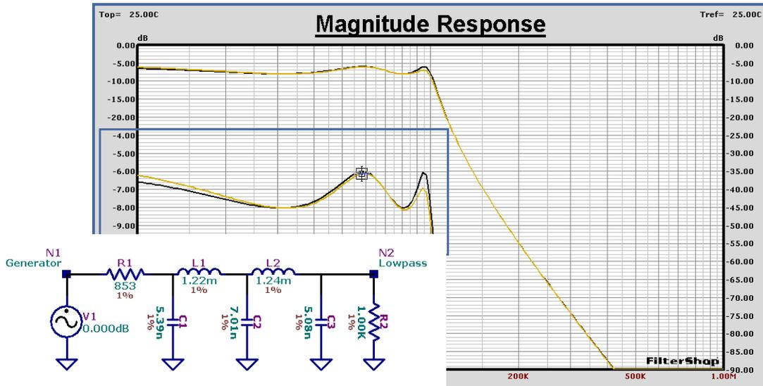
An examination of the sensitivity shows a worst case value of about 3, for C2 as shown below. This is about what would be expected for a sharp Chebyshev type response. If a smoother target function had been selected the sensitivity values would have been reduced.
