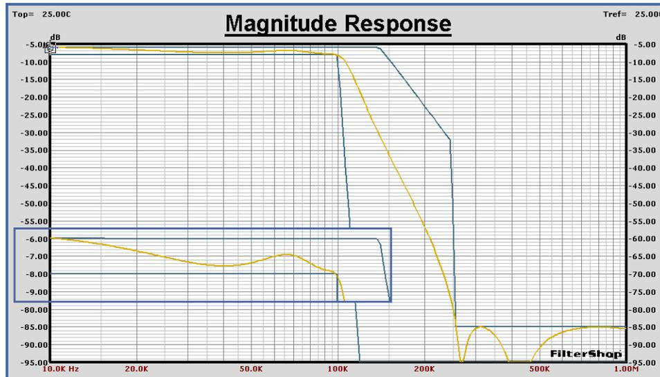
If we now select 5% precision for the capacitors and inductors, the schematic and response shown below are produced. Both the passband and stopband are only slightly changed.
