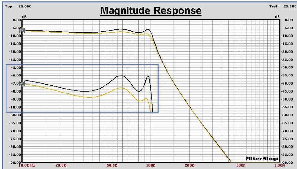
As before we can attempt to optimize the circuit with loss to the original target response. After this is done, the response curve is shown below.
