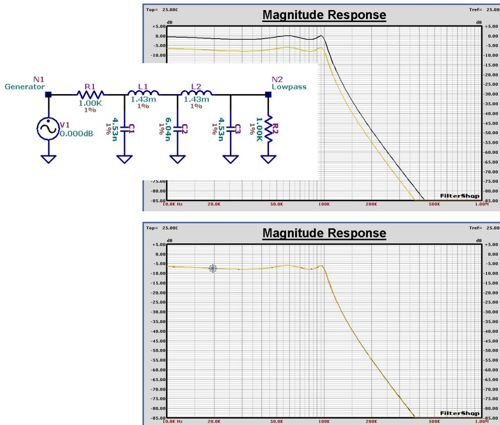
Synthesis produced equal values for both L1 and L2 of 1.43mH. However, the inductors are currently being modeled as virtually lossless. The default series resistance is 1u Ohm and the default shunt capacitance is 1f Farad. The equivalent circuit for the inductor is shown below.
