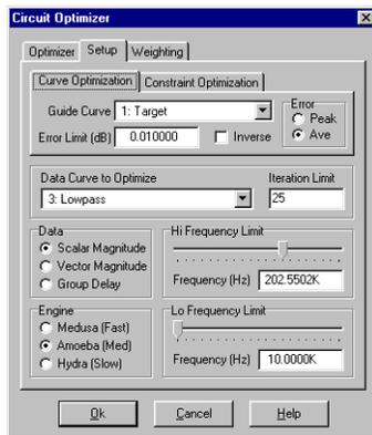
The circuit optimizer setup is shown here, along with the final result shown below. R1 has decreased as expected. Both of the inductors have dropped in value slightly, and the capacitors have increased.
