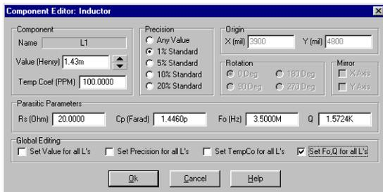
We first enter the  $F_o$  frequency at 3.5MHz. This calculates the  $C_p$  value for us. Next we enter the  $R_s$  value of 20 Ohms. This updates the  $Q$  as 1500. We also enable the *Set  $F_o/Q$  for all Inductors* to copy the changes to  $L_2$  as well.
