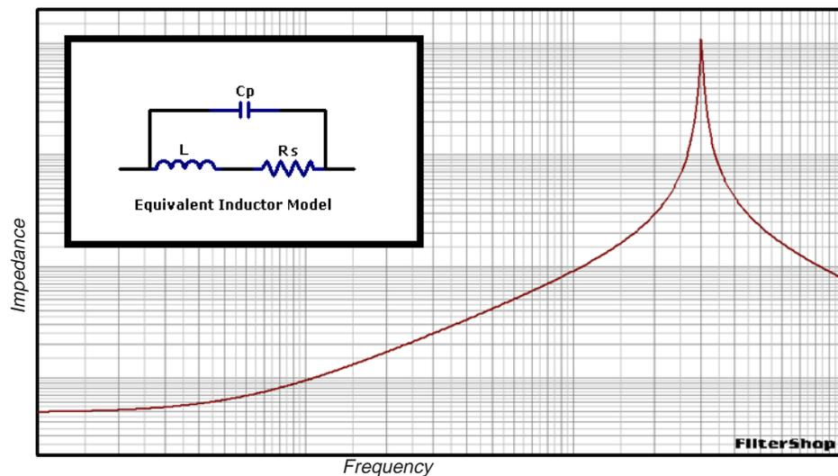
To model the losses in the inductors, we need to change the values of Rs and Cp for L1 and L2 into something more realistic. One way to approach this is to examine an actual catalog listing for parts that could be used. An axial half inch size inductor in this value range was found to have the following specs:
