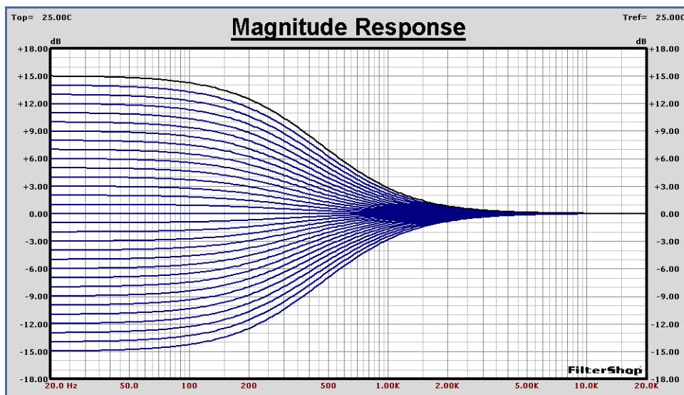
*HEQ and HEQ<sup>2</sup> Filter Functions, F<sub>o</sub>=300Hz
