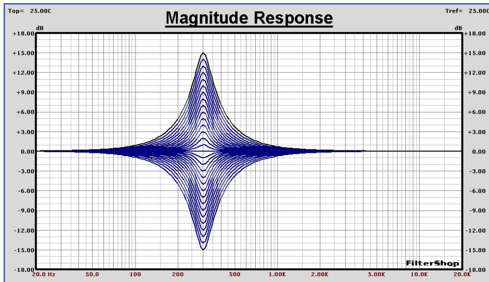
*BEQ Filter Functions, Ao=+15dB, Fo=30Hz...300Hz, Oct=3.0...0.333
